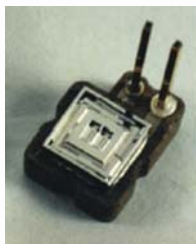
Test devices: micro pumps (source: IZMM), HT-EEPROM (source: IMS), integrated surface micromachined pressure sensor on SOI (source: IMS)
