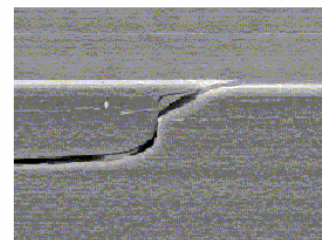
Cracks in single crystal silicon support beams caused by vibrations induced by a launch simulation (source: CSL)
