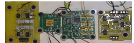
Injection of test signals into bias structures to test magnetometers
